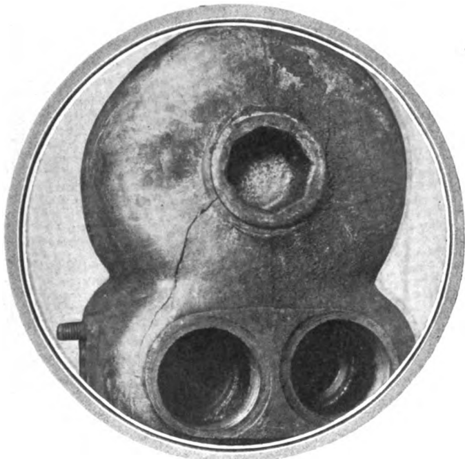
Fig. 3—Showing a cracked water jacket which will allow the cooling water to run away
